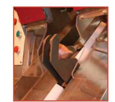
This system offers a complete process for 45mm to 115mm diameter onions. It tops and tails the onions in one operation then slits the outer skin and removes it with compressed air. No change parts are required.
