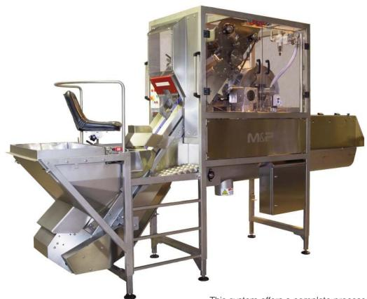
This system offers a complete process for 45mm to 115mm diameter onions. It tops and tails the onions in one operation then slits the outer skin and removes it with compressed air. No change parts are required. The onions are picked up from the hopper automatically and then positioned by the feed operator so that the tops and tails are set horizontally across the carriers.
