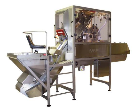
This system offers a complete process for 40mm to 90mm diameter shallots It tops and tails the shallots in one operation then slits the outer skin and removes it with compressed air. No change parts are required. The shallots are picked up from the hopper automatically and then positioned by the feed operator so that the tops and tails are set horizontally across the carriers.
